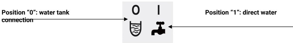
**4.3.1 Machine in use with direct water connection**
