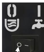
Place switch into position "0" when operating machine with water tank
